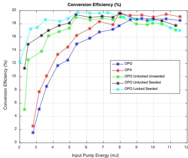
Figure 9-3. Conversion efficiency correspond to figure 9-2.
