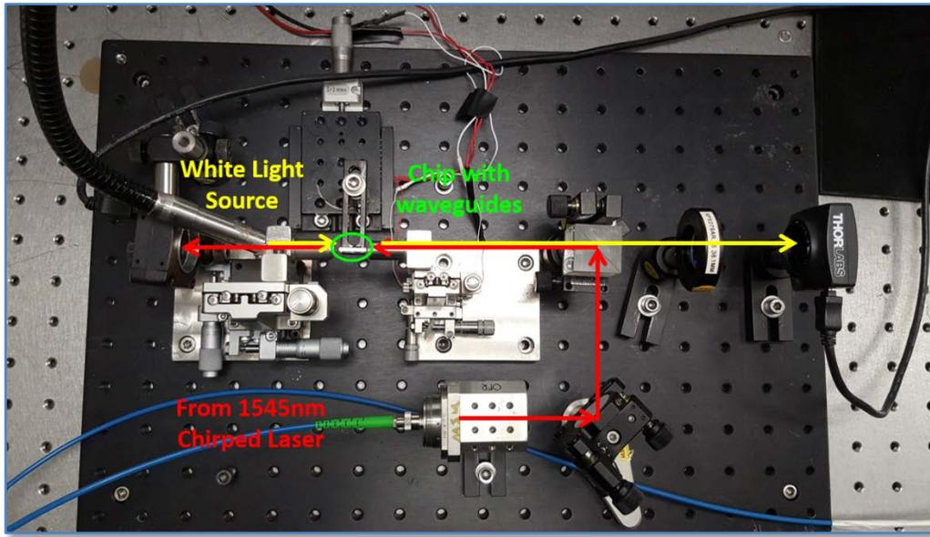
Figure 8-8. Added components for assisting in alignment and coupling light into waveguides include a white light source, a beam splitter designed for visible light, a lens, and a visible light camera. The beam splitter acts like a mirror to the 1545 nm laser light. The input coupling lens and the new lens form a telescope. The white light source and the camera provide visualization of the waveguide chip front facet.
