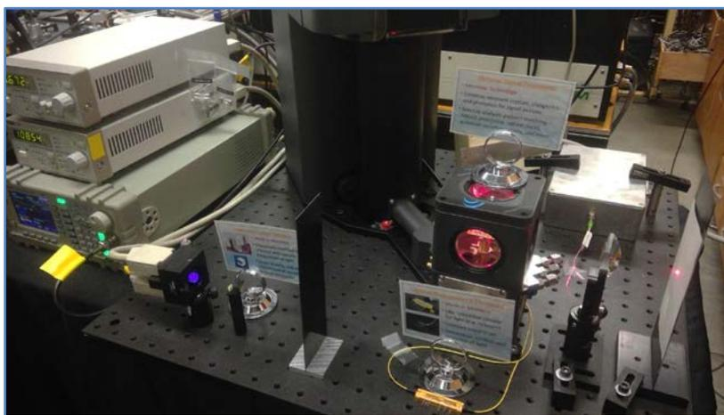
Figure 8-11. Demonstration system constructed to illustrate integration of Montana Instruments Cryostat with AdvR Inc waveguides, Scientific Materials Corp. crystals, and S2 Corp photonic signal processing.
