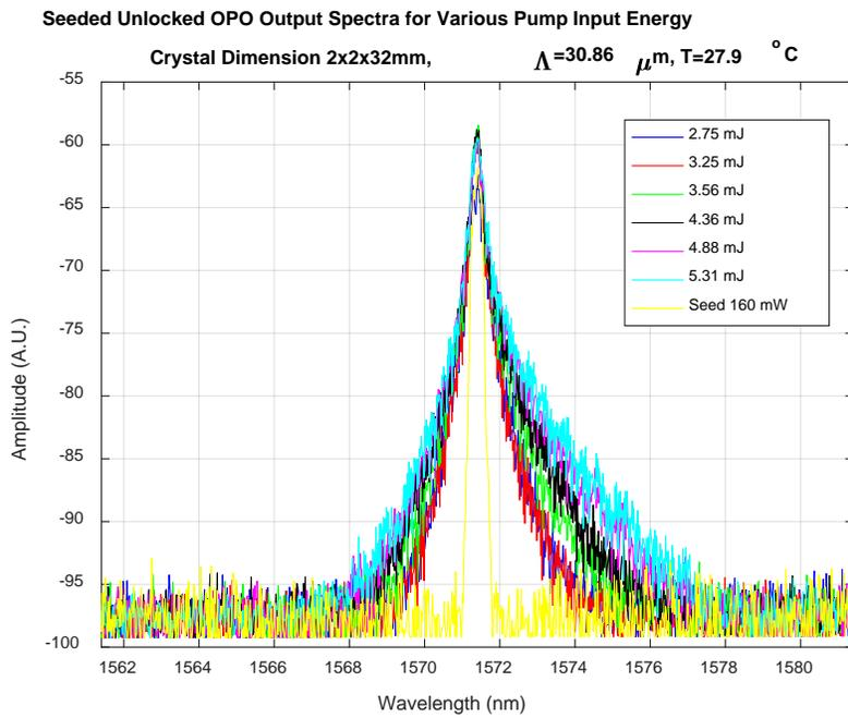
Figure 9-7. Output spectra for seeded-unlocked OPO.
