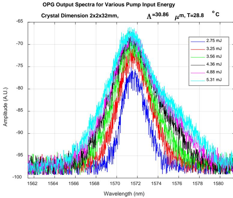
Figure 9-4. Output spectra for OPG.
