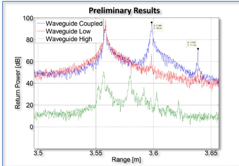
Figure 8-7. Post processed signals from the balanced detectors. The blue signal is a correctly coupled into a waveguide result. The green and red signals are results of the chirp laser signal being above the waveguide and below the waveguide yet in the substrate, respectively. The coinciding peak of the coupled and low signals refers to the front facet of the waveguide chip. The next two peaks in the coupled signal correlate to the first and second reflections off of the waveguide back facet.
