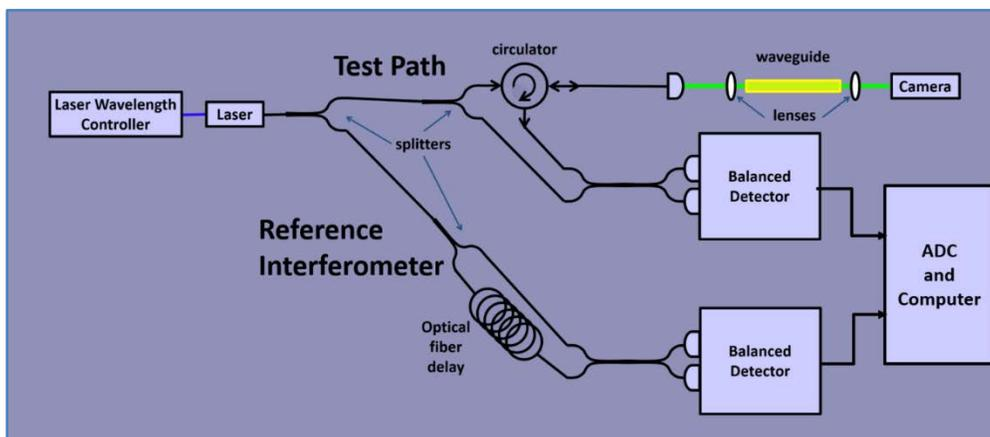
Figure 8-4. Test Setup for nondestructive optical waveguide characterization. An ultra-high resolution FMCW lidar signal is split between the optical waveguide path and a reference interferometer path. The interferometer signal is used in post processing to remove any nonlinearities of the laser chirp modulation. This method of determining waveguide propagation loss is independent of input and output coupling losses.
