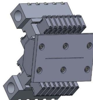
Figure 2-2. Airjet manifold for sorting system.
