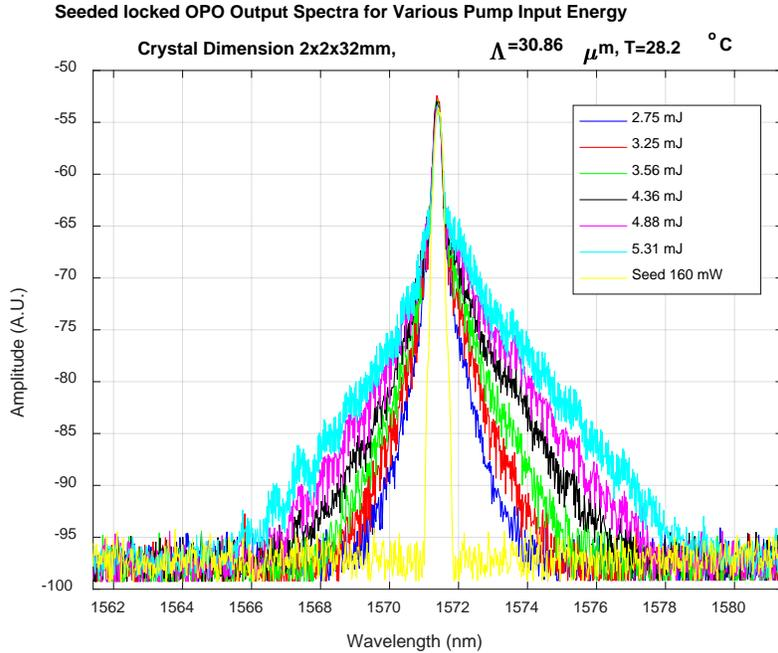
Figure 9-8. Output spectra for seeded-locked OPO.
