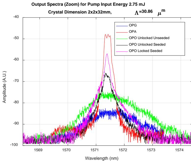
Figure 9-9. Output spectra for OPG/OPA/OPO with 2.75 mJ input pump energy.
