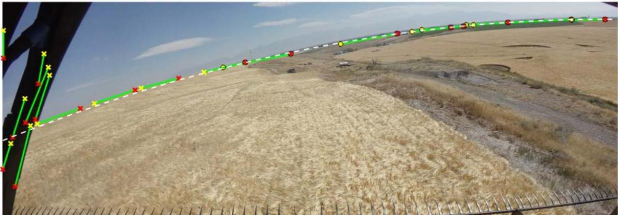
Figure 1-6. Image processing for horizon detection used in mask adjustment of hill imagery.
