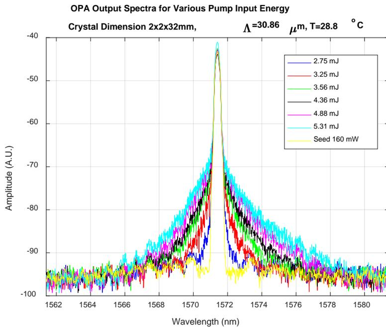
Figure 9-5. Output spectra for OPA.
