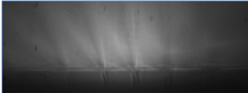
Figure 8-9. Camera image of the waveguide chip top front facet showing a few waveguides.
