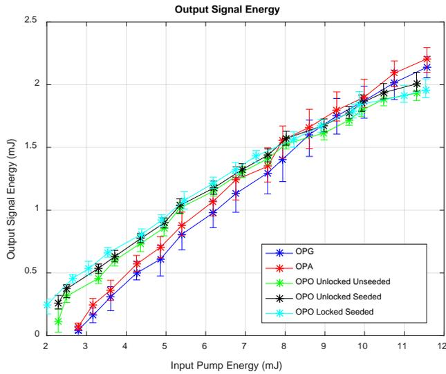
Figure 9-2. Output signal energy for OPG/OPA/OPO cases
