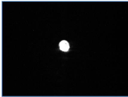
Figure 8-6. A guided optical mode captured on camera.
