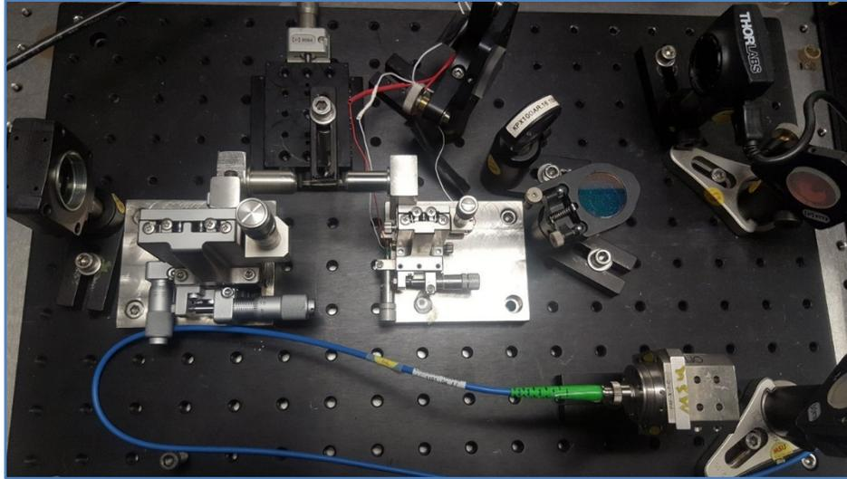
Figure 8-5. Photo of test path free-space section. The waveguide chip is positioned between two xyz-stages using an x-stage. A camera is used to image the coupled optical mode.
